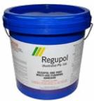
**Regupol One Part Multi-Use Flooring Adhesive** is a water based synthetic polymer, VOC compliant, multi-use flooring adhesive, with water resistant properties. This adhesive was specifically formulated to bond selected Regupol® products to most common interior sub-floors. The product is suitable for dry area installations only.
