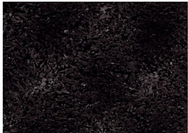
Regupol® 6010 is manufactured using recycled SBR rubber
