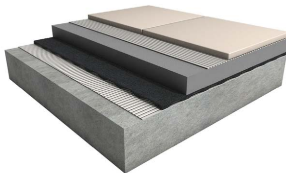
Typical bonded screed bed system with tiled floor - dry area - includes approved Regupol adhesives. Refer to under screed flooring acoustic system for more technical information.
