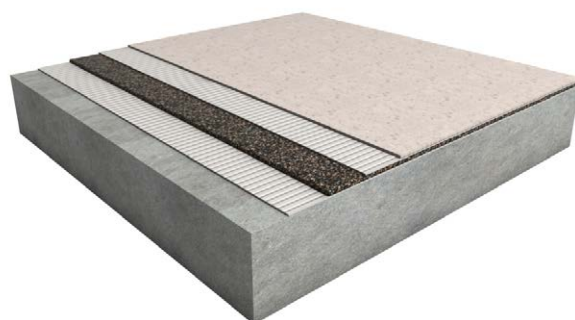
Typical resilient floor system includes approved Regupol adhesives. Refer to resilient flooring acoustic system for more technical information.
