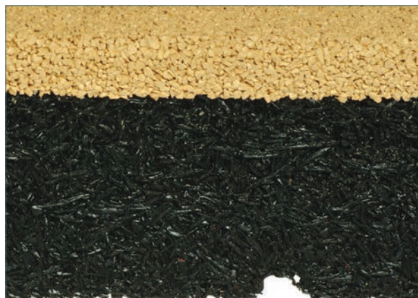
The cross section shows the dual-layer construction with the solid-coloured EPDM layer.
