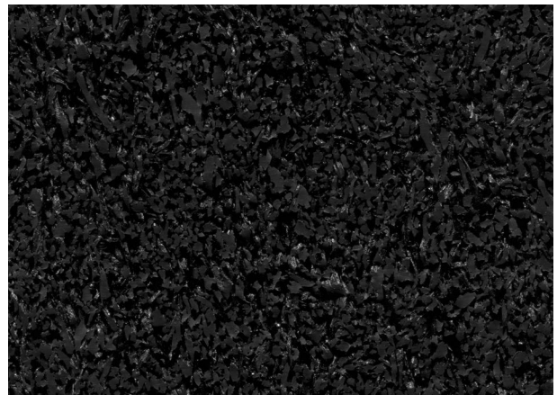
Regupol® 6010 10mm impact sound acoustic underlay
